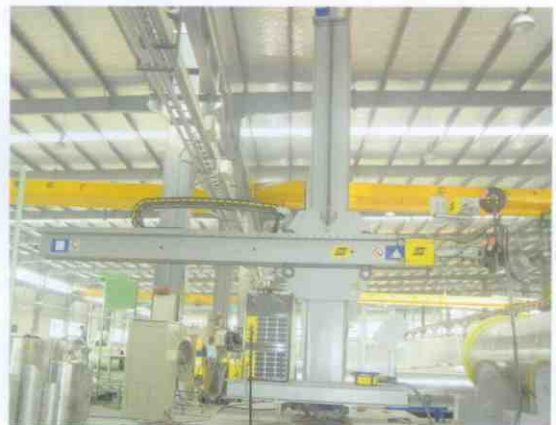
进口全自动环缝焊接工作站(瑞典) The Fully Automatic Ring-seam Welding Station (Imported from Sweden)
