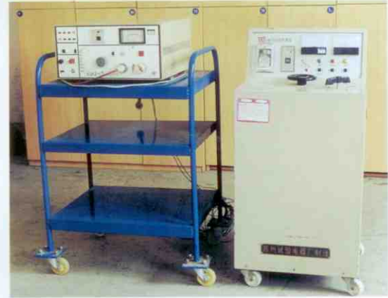
耐压试验设备 The Withstand Voltage Test equipments
