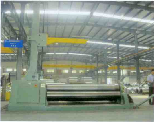
进口全自动微机控制4辊卷板机(瑞典) The Fully Automatic Micro-processor Control Bending Machine with 4 Rollers (Imported from Sweden)
